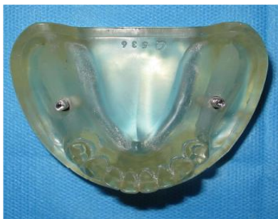
Figure 3. Photoelastic model of mandible with implants placed in edentulous areas
