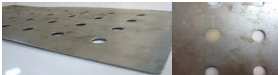
Figure 1: Disc-shaped moulds for fabrication of solubility testing specimens
